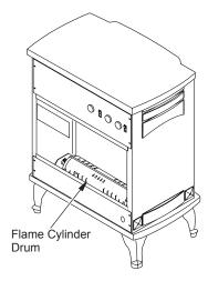
Figure 7 - Flame Cylinder Drum Location
